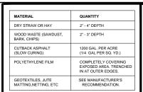
STRAW OR HAY MULCH SHALL BE ANCHORED IMMEDIATELY AFTER APPLICATION. MULCH MAY BE ANCHORED BY MECHANICALLY PRESSING INTO SURFACE. IF SPREAD WITH BLOWER EQUIPMENT, MULCH SHALL BE ANCHORED WITH MULSIFIED ASPHALT (GRADE AE-5 OR SS-1)-100 GAL. ASPHALT + 100 GAL. WATER PER TON OF MULCH. POLYETHYLENE SHALL BE TRENCHED IN AT EDGES.
